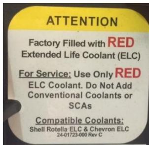
**Propane** equipped units will be using a different product designed for gas engines. It is maintained in the same fashion as the OAT coolant, being certain not to mix it with other coolants and use the proper makeup fluids.
